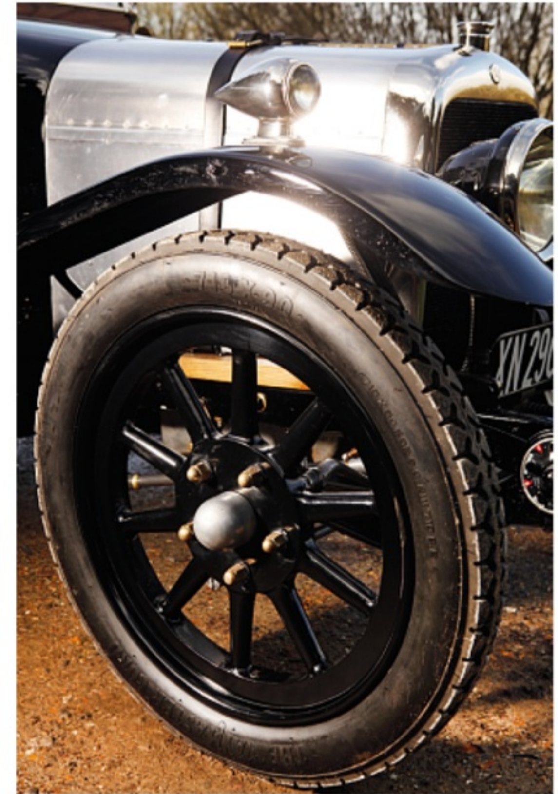
Clockwise: single-carb sidevalve 'four' musters 40bhp, but A3 struggles up hills; charming chassis plate; 'Sankey' wheels recreated in aluminium
