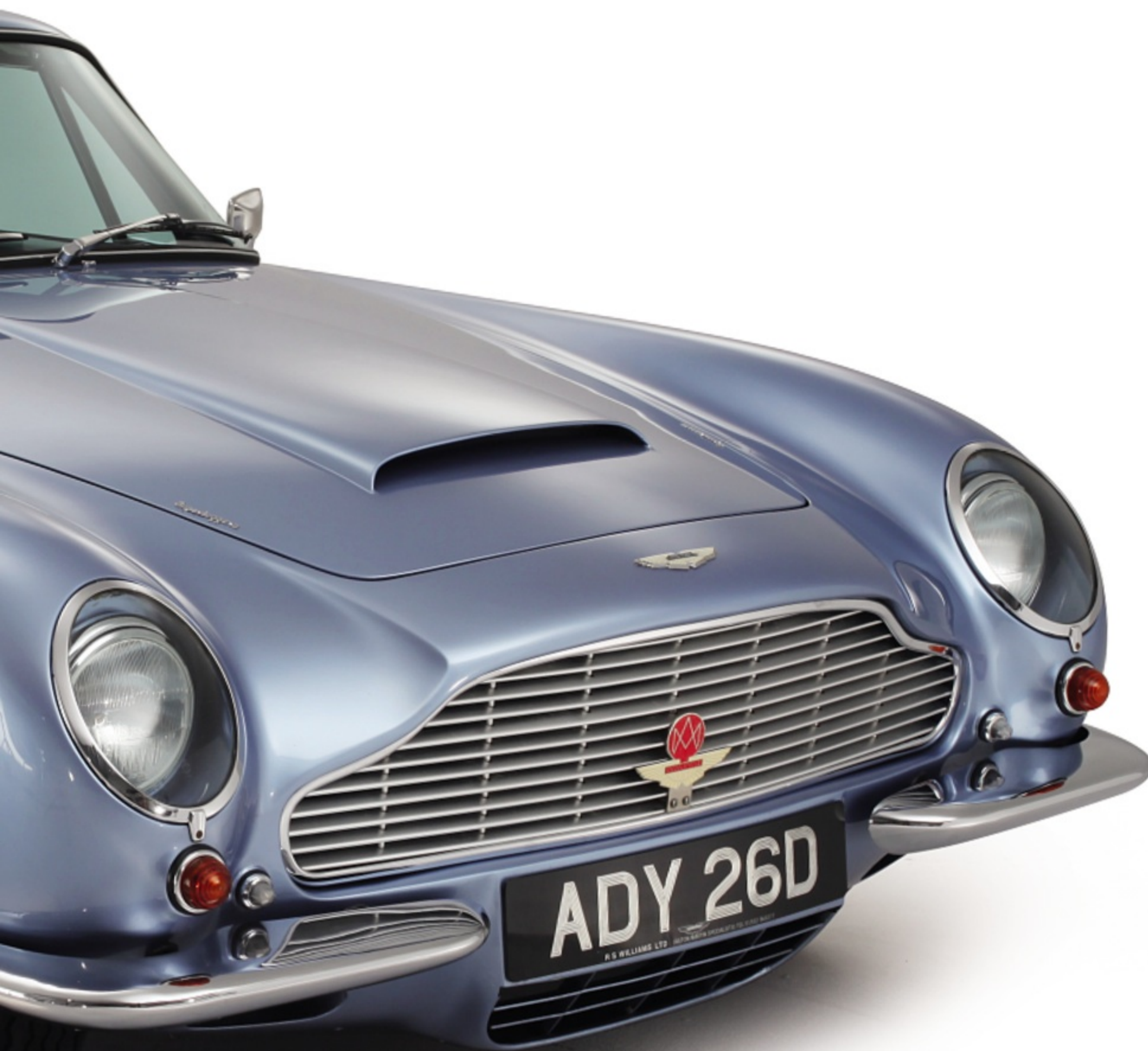
Above: Mk2's lipped arches allow for wider rubber than Mk1 DB6, and quarter-bumpers flank the extra grille. Below: luxurious DB6 is a full four-seater
